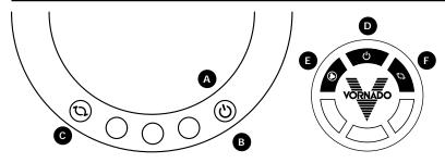
**Flippi V Power** (A) The unit functions ON and OFF by pressing the POWER button. Lights on the unit's control panel indicate the power is ON.
