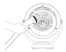
To clean motor cap and inlet ribs: Use a common household vacuum. Do not use water to clean these parts of the Air Circulator.
