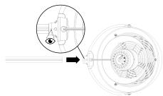
**6.** With circulator still resting on soft surface, insert lower pole into recess on top of base. From underside of base, fully tighten thumb screw to secure.
