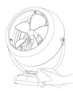
To clean blade: Wipe with a damp cloth. If your Air Circulator is used in a greasy environment, such as a kitchen, mild soap or a common household cleaner may be necessary. Do not use solvents.
