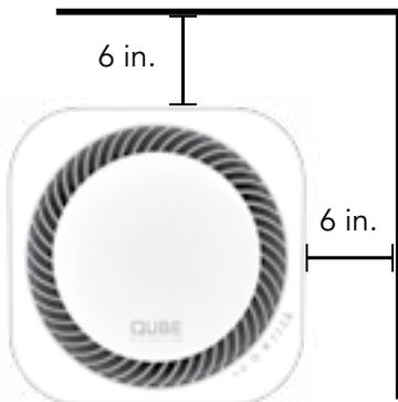
**Note:** For optimum airflow, air outlet should be unobstructed. Ensure curtains and other items are far enough away from the unit to not be pulled into the side inlets or interfere with airflow.
