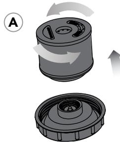
4. Install new Cartridge onto Cap.
